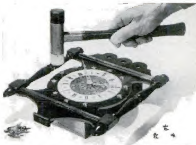
STARS AROUND DIAL are lightly tapped into pre-drilled holes located on 6 1/2-in.-dia. penciled circle
